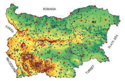
Fig. 1. The present NIMH weather stations network: synoptic (squares), climatological (triangles) and rain-gauge (circles) stations.
