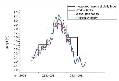
Fig. 5. Comparison of the measured daily maximum surge measured at Irakli tide gauge with model simulations for the storm of January 1998 using the default Smith-Banke formula and  $C_d$  estimated using the wave steepness and  $C_d$  based on the friction velocity obtained by the SWAN wave model.
