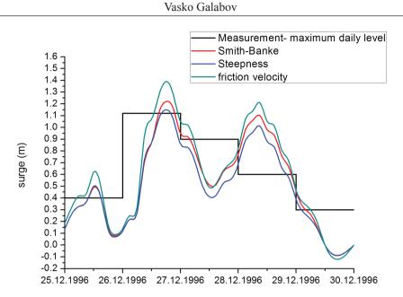
Fig. 4. Comparison of the measured daily maximum surge during the storm of December 1996 measured at Ahtopol tide gauge with model simulations using the default Smith-Banke formula and  $C_d$  estimated using the wave steepness and  $C_d$  based on the friction velocity obtained by the SWAN wave model.
