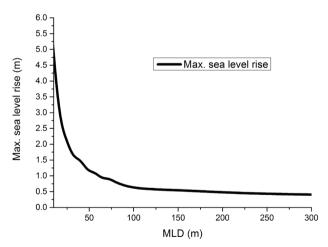
Fig. 1. Dependence of the maximum sea level rise of the depth of integration for the storm of February 1979
