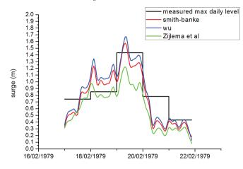
Fig. 2. Comparison of the measured daily maximum surge measured at Irakli tide gauge with model simulations using Smith-Banke and Wu bulk parameterizations of  $C_d$  and the second order bulk formula of Zijlema et al (2012).
