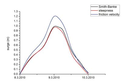
Fig. 6. Model simulations using the default Smith-Banke formula and  $C_d$  estimated using the wave steepness and  $C_d$  based on the friction velocity obtained by the SWAN wave model- the storm of March 2010.
