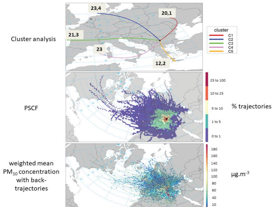
**Fig. 9.** Cluster analysis, PSCF and weighted mean  $PM_{10}$  concentration with back-trajectories for Sofia
