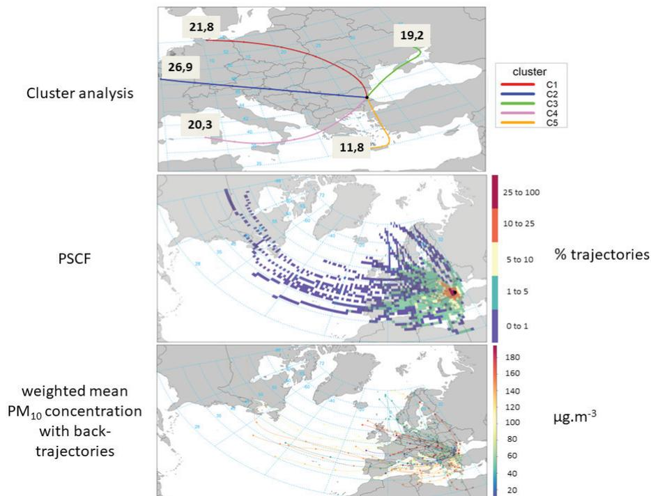
**Fig. 8.** Cluster analysis, PSCF and weighted mean  $PM_{10}$  concentration with back-trajectories for Burgas
